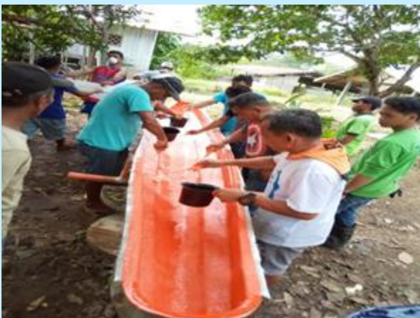
Hands-on training on fiberglass reinforced plastic (FRP) boat fabrication under the SAAD Program in La Paz, Loreto and Talacogon, Agusan del Sur.
