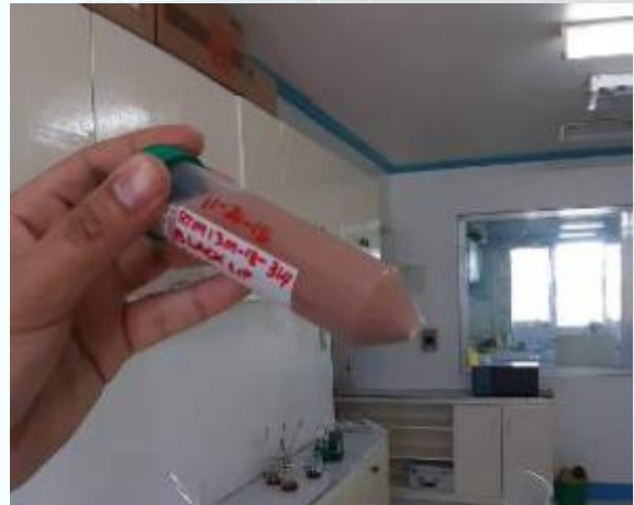
A sample of shellfish meat (Black Lip) prepared by acid extraction. The sample was sent to the BFAR National Fisheries Laboratory Division for confirmatory tests (MBA or RBA).
